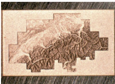
FIGURE 6: Micro-structured copper plate (circa 9 mm wide) using topographical data from the Swiss Federal Office of Topography swisstopo ( www.swisstopo.ch ) used with permission geodata@swisstopo . Photo and sample preparation courtesy of Prof. B. Neuenschwander, Bern University of Applied Sciences.
